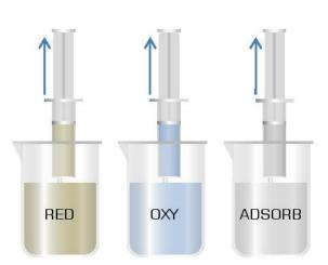
5. Load the prepared solution in the provided syringes. Make sure to use separate syringes for each chemical. The loading amount should be noted to realize the performance.
