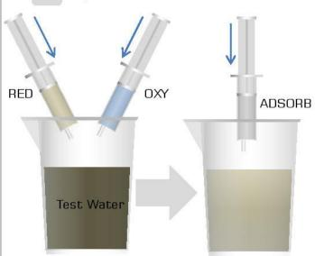
6. Put 1 liter of test water in the plastic mug and inject RED & OXY simultaneously with both hands. Stir the mixture for 1 minute. Add ADSORB to the mixture and stir for 1 minute. Leave the solution in rest for 10. minutes.
